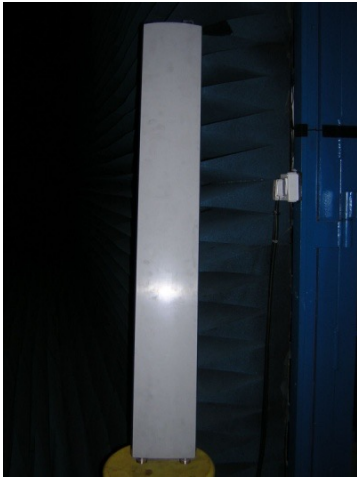
UMTS antenna (1920 MHz)
